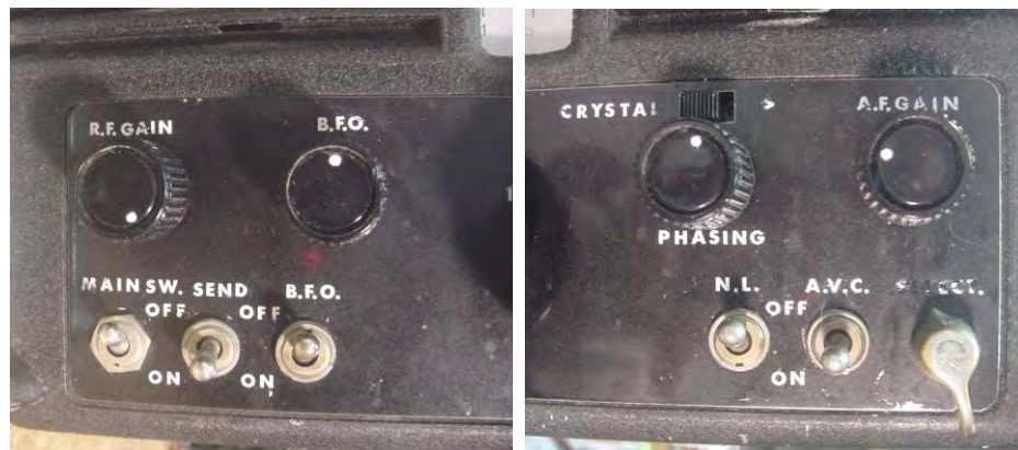
Above: detail of the fingerplate lettering (white Letraset on black paint) and mongrel small knobs fitted to the S.680/2 on arrival at my shack – functional? er, yes, authentic-looking? er, not exactly...
