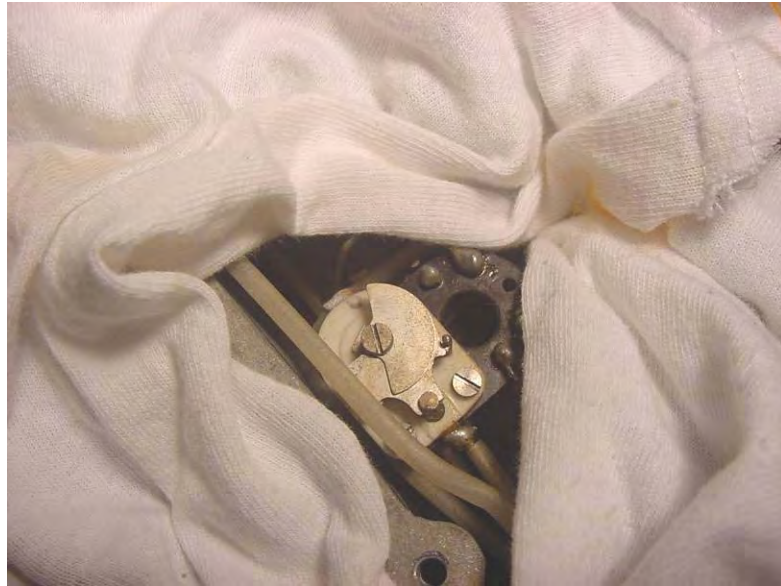
Careful shrouding of the surrounding trimmers when cleaning out debris from the slug
