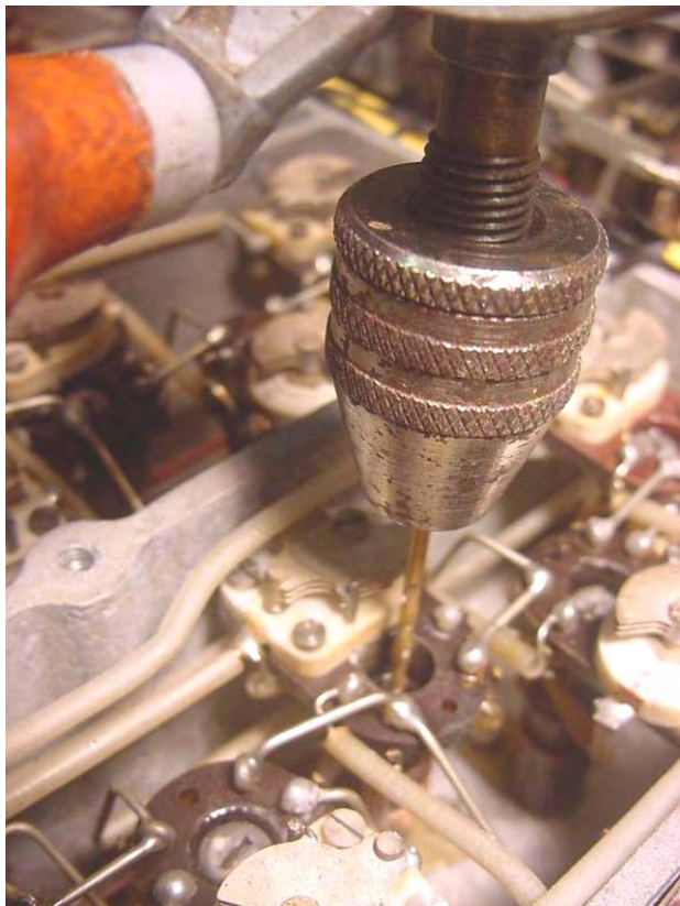
Drilling the centre of the broken or stuck slugs
